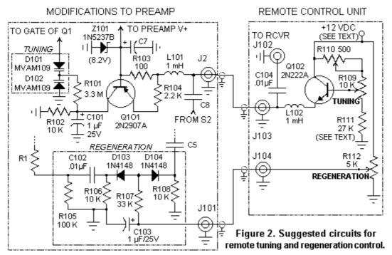
If you want, you can run a multiple-conductor shielded cable between the control unit and preamp, and use separate wires for power, signal and tuning. (I've used 150 feet of ordinary audio cable in my field tests of the preamp with no significant loss of signal.) Separate wires let you use a much simpler remote tuning circuit. But that's too easy. Figure 2 shows how to make one shielded wire perform multiple tasks. Q101 functions as a DC amplifier with offset, so that the tuning voltage varies
